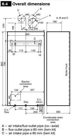
Fig. 6.2 (all dimensions in mm)
