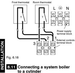
Two schematic wiring diagrams are given in this section showing two possible ways to connect an external programmer to a mid-position diverter valve to provide independent timed and thermostatic control of heating and hot water.
